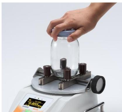
Torque measurement of PET bottle caps
