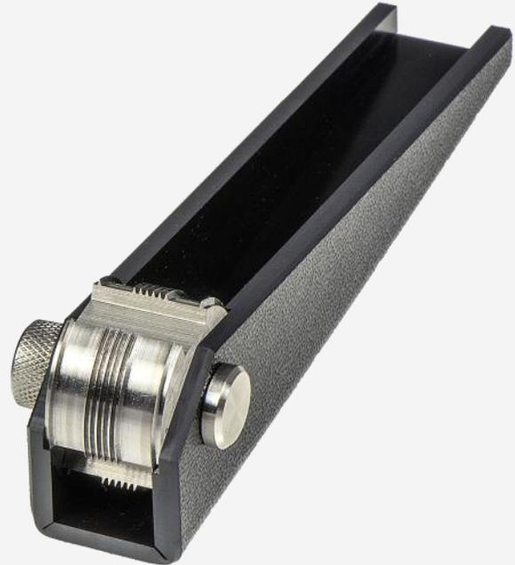
Repeat this operation making further parallel cuts, crossing the original cuts at 90° so that a lattice pattern is formed.
