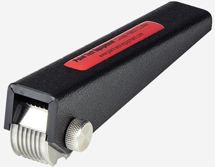
The coating thickness determines the Cutter size used.
