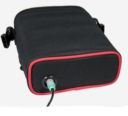
The Holiday Detector earth cable must have a secure connection to the substrate of the item under test.
