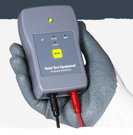
Connect the Earth Cable to the base metal of the item under test. It is essential that the base metal of the item being tested is also connected to a true earth
