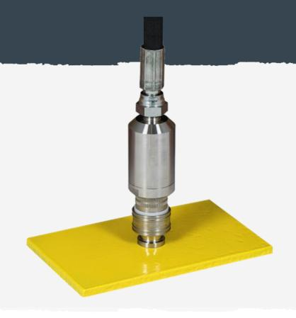
Check that no adhesive has been left in the dolly hole by trial fitting the Dolly Plug.
