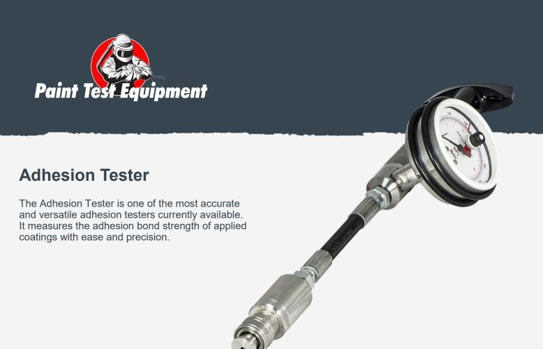
The adhesion is measured by the tensile pull on a Dolly glued to the coating surface. The force is applied through the centre of the Dolly by a hydraulically loaded pin. This ensures an exactly central point-loading of the force.
