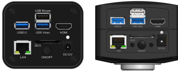
Figure 2 Available Ports on the Back Panel of the Camera Body(Cubic and Flat Shape)
